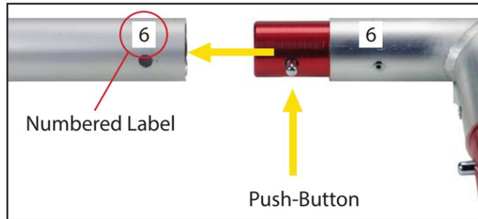
Connections are made by holding the button down and sliding the red tube into opposing tube until it locks in place. To disassemble push button and pull or twist extrusions apart.
